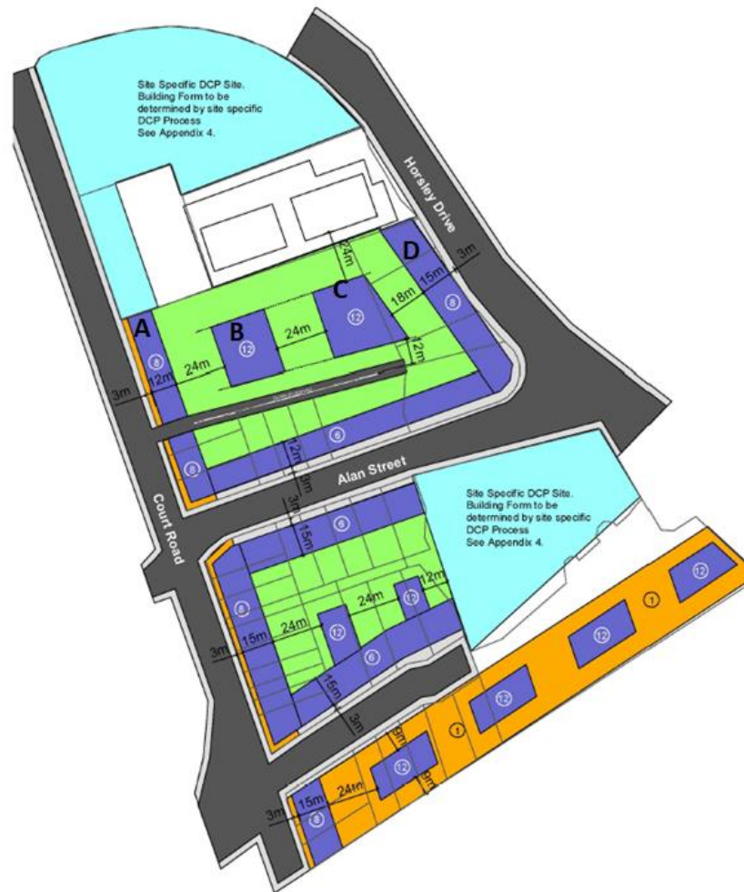
Figure 5: Fig 4.7-3 Court Road Precinct– Plan View and Permitted Building Height (Source: Fairfield City Centre DCP 2013).
